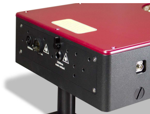
Switchable output of the TEMA-DUO-100 femtosecond laser (fundamental only or simultaneous fundamental and SHG)
