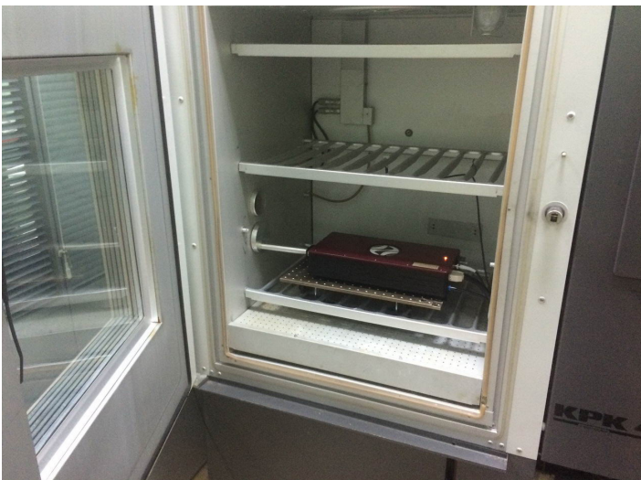
Thermal cycling of a TEMA system within 10...40 °C temperature span
