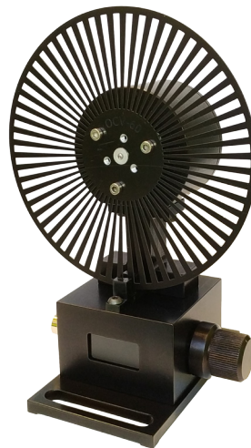
The OCV-6300F optical chopper with a 60-slot blade
